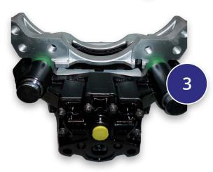
Place end caps over guide pins and tap in with a hammer.
