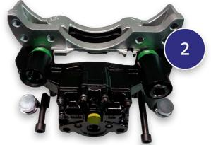
Place cradle into the caliper. Apply thread lock glue to the threads of the bolts.
